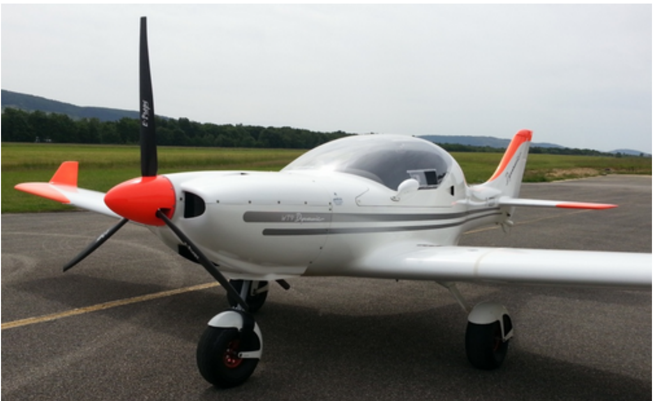
towing ultralight WT9 Dynamic, Rotax 912S, E-Props Durandal 100-R propeller
