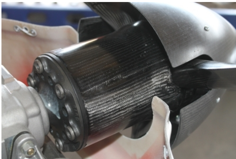
extended hub on a ROTAX's reducer with a spinner
