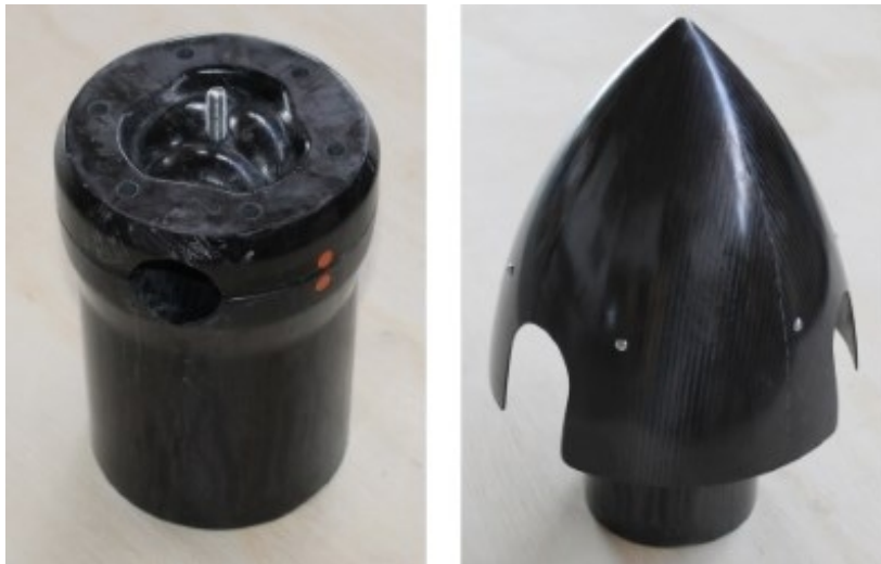
hub with integrated spacer 115 mm (for Savannah, for example) and on the right with a 250 mm spinner
