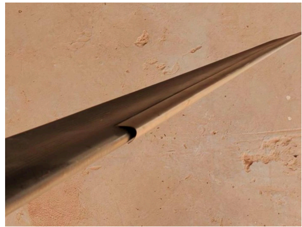
Fig. 2 – Detail of the debonded leading-edge protection
