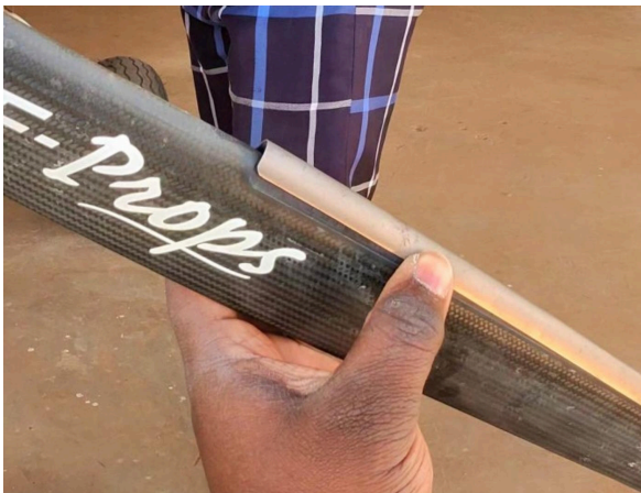
Fig. 1 – Blade with leading-edge protection detachment
