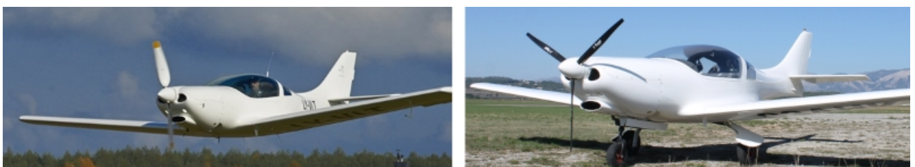
wide blades or thin blades? the thin ones generate much less drag, and therefore increase efficiency...
