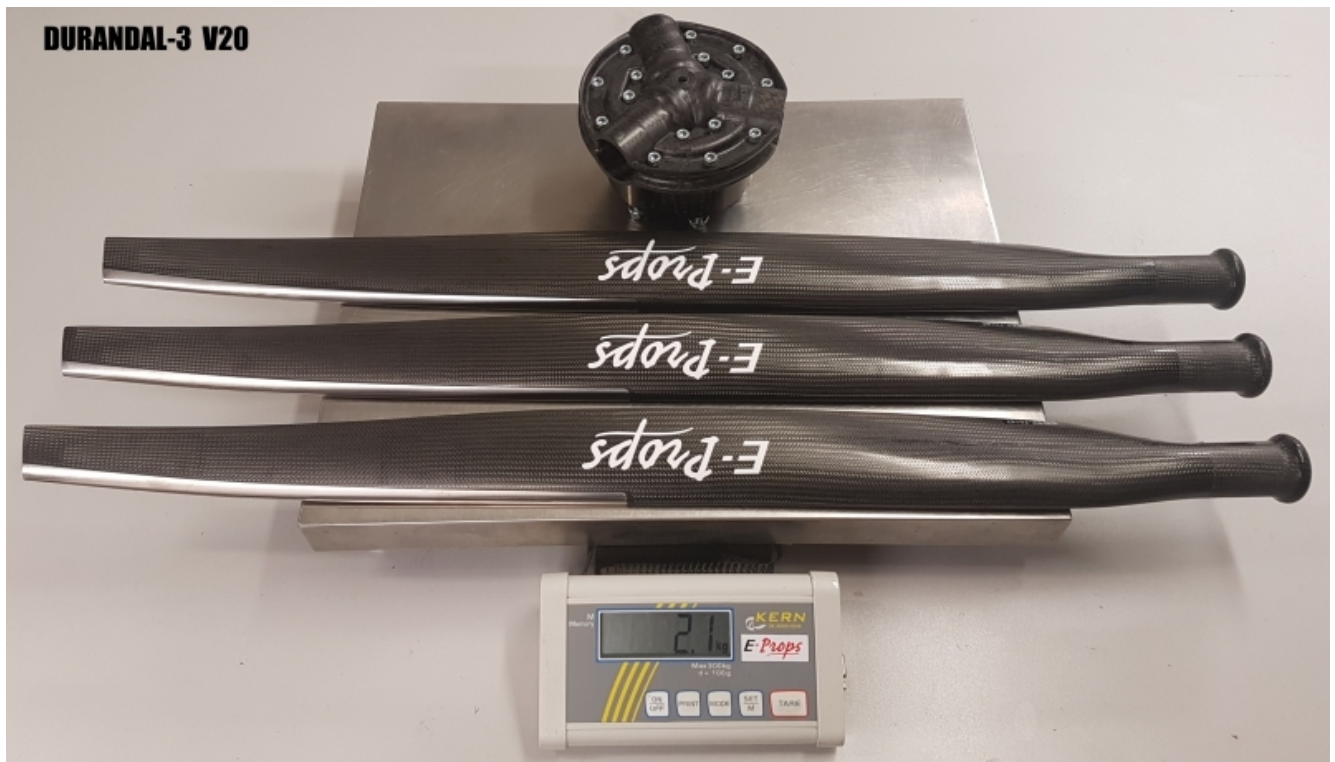
3-blade DURANDAL-3 diameter 170 cm, Titanium leading edge protection, with all screws = 2,1 kg
