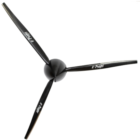
Durandal : ground adjustable pitch
