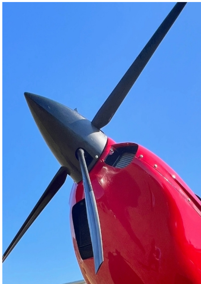
E-Props 4-blade propeller diameter 203 cm
