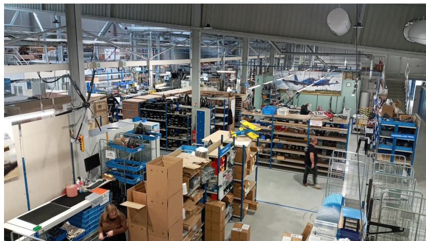
Final assembly area of the E-Props workshop, tracked in real time by RFID and KANBAN
