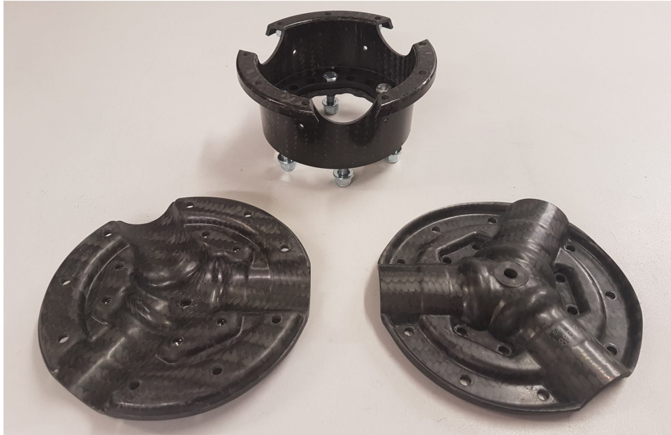
The three components of a hub, plus a spacer, for a 3-blade propeller
