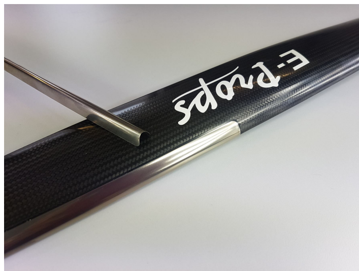
Titanium leading-edge shield bonded onto the carbon blade
