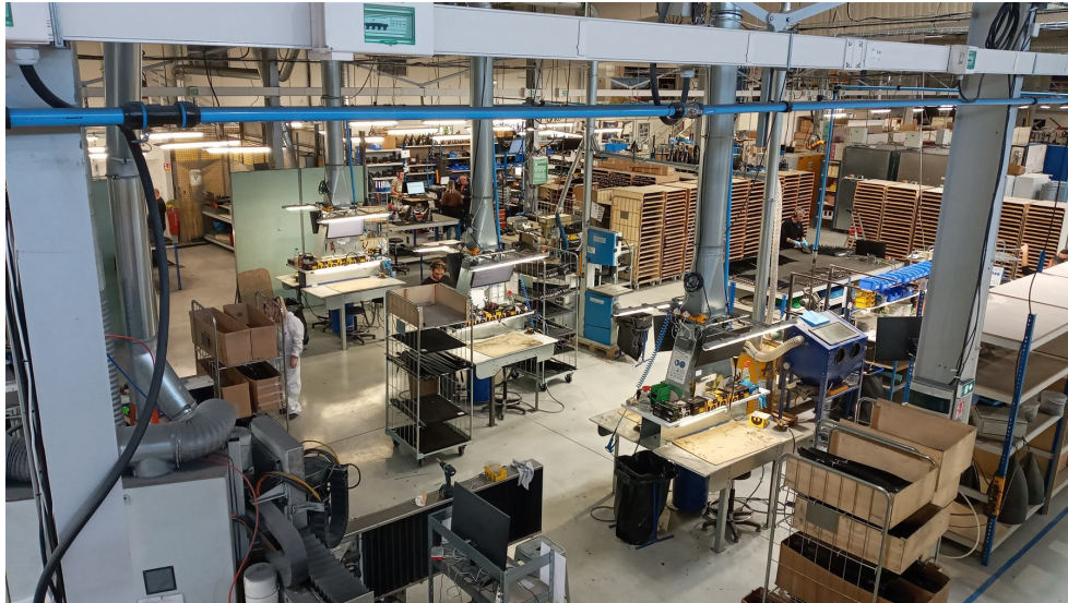
Production floor: mold storage, CNC finishing and RFID-tracked work-in-progress
