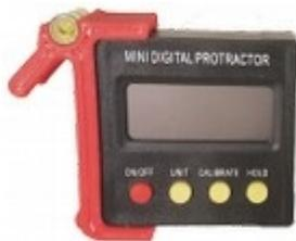
*Digital protractor (precision :  $\pm 0,1^\circ$ )*
