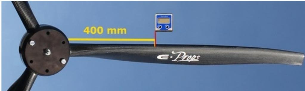
Trick : put some tapes at 400 mm of the side of the hub (do not forget to remove them before to go flying !).
