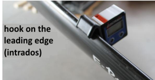
E-PROPS propeller blades have a quite curved leading edge and an important dihedral. These two data request that pitch measurement must be carried out with blades exactly in the same place.
