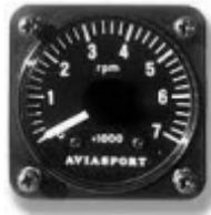
If the propeller is fixed pitch, the propeller manufacturer will have to make the propeller corresponding to the indications of the tachometer, and not to the real engine parameters. This is a frequent occurrence.
