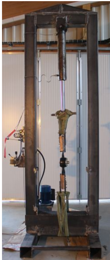
carbon hub + Vorpaline blade on a bench test with instruments
