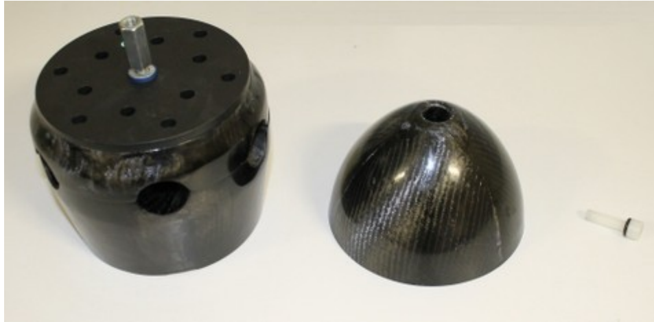
hub with long screw + Nord-Lock washer Mini-Spinner + Nylon screw + seal
